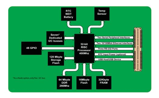
FIGURE 2. VT002 Functional Block Diagram
